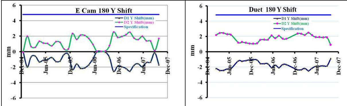
**Fig 9:** The Y Shift result for detector 1 (D1) and detector 2 (D2) in Ecam camera with 180 configuration degrees through 30 months.
