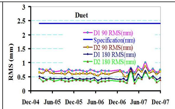
**Fig 8:** The root mean square (RMS) in mm for detector 1 (D1) and detector 2 (D2) in Duet camera with 180 and 90 configuration degrees through 30 months.
