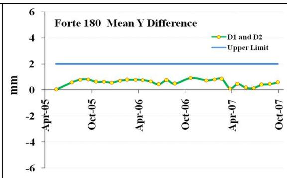
**Fig 16:** The Mean Y Shift result for detector 1 (D1) and detector 2 (D2) in Forte camera with 180 configuration degrees through 26 months.
