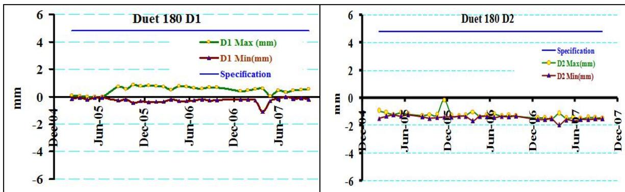
Fig 5: MHR/ COR calibration result of X- Maximum, X- minimum and specification for detector 1(D1) and detector 2 (D2) in Duet camera with 180 configuration degree through 30 months.
