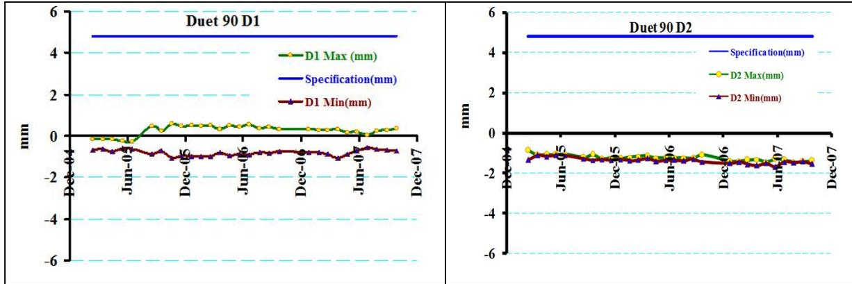
**Fig 6:** MHR/ COR calibration result of X- Maximum, X- minimum and specification for detector 1(D1) and detector 2 (D2) in Duet camera with 90 configuration degree through 30 months.
