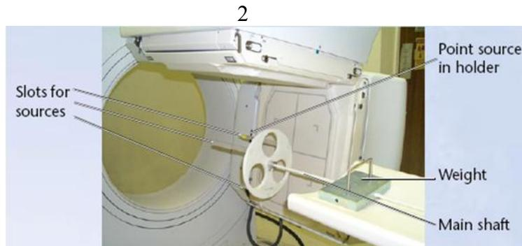
**Fig.2:** Point sources assembly used with Philips (Forte) gamma camera.
