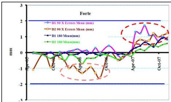
**Fig 15:** The X errors mean for detector 1 (D1) and detector 2 (D2) in Forte camera with 180 and 90 configuration degrees through 26 months.
