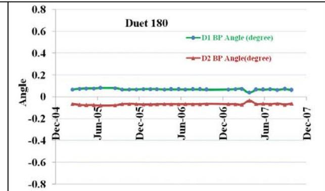
**Fig. 12.** The Back projection angle result for detector 1 (D1) and detector 2 (D2) in Duet camera with 180 configuration degrees through 30 months
