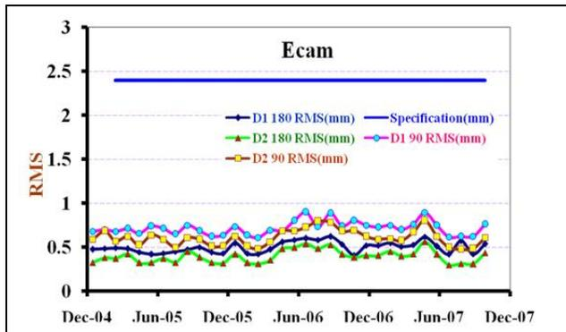
**Fig 7:** The root mean square (RMS) in mm for detector 1 (D1) and detector 2 (D2) in Ecam camera with 180 and 90 configuration degrees through 30 months.
