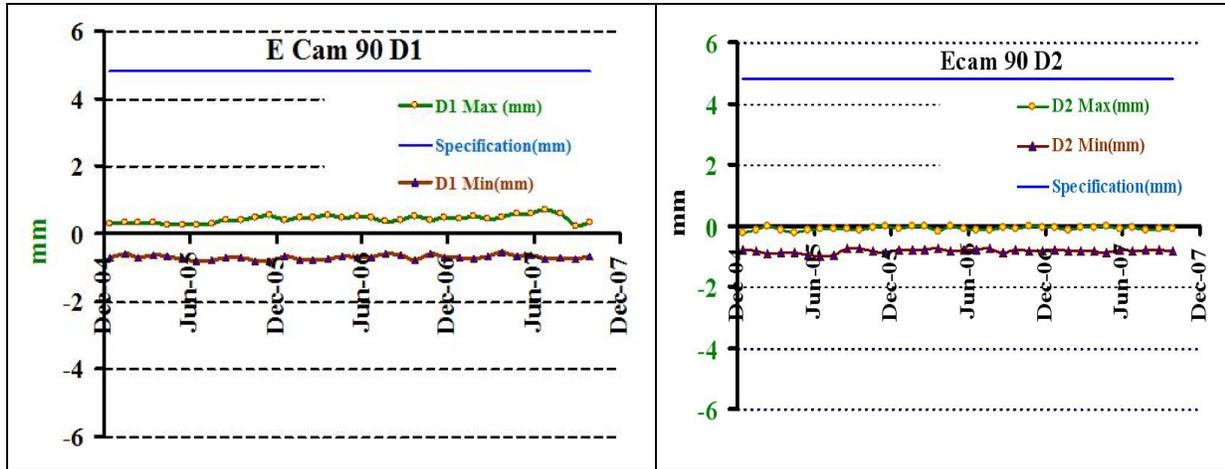
Fig 4: MHR/ COR calibration result of X- Maximum, X- minimum and specification for detector 1(D1) and detector 2 (D2) in Ecam camera with 90 configuration degree through 30 months.
