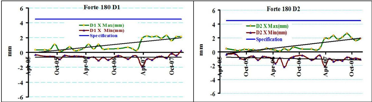
**Fig 13:** COR QA result of X- Maximum, X- minimum and specification for detector 1(D1) and detector 2 (D2) in Forte camera with 180 configuration degree through 26 months. The solid line is the statistic trend line for the result.
