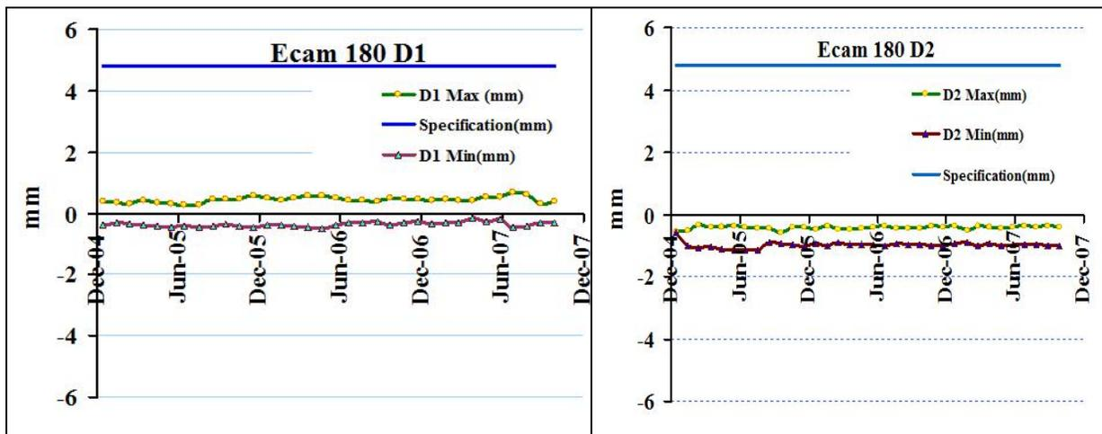
**Fig 3:** MHR/ COR calibration result of X- Maximum, X- minimum and specification for detector 1(D1) and detector 2 (D2) in Ecam camera with 180 configuration degree through 30 months.
